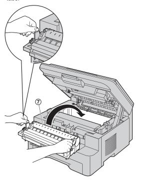
• Make sure that the triangles (®) match, to install the drum and toner unit correctly.
